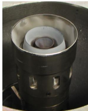
Fuel (natural gas) is injected 295 mm upstream the burner nozzle.
